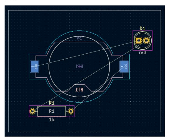
All PCB layers are viewed from front side of the board. Footprints on the bottom of the board are therefore upside down and appear mirrored.
